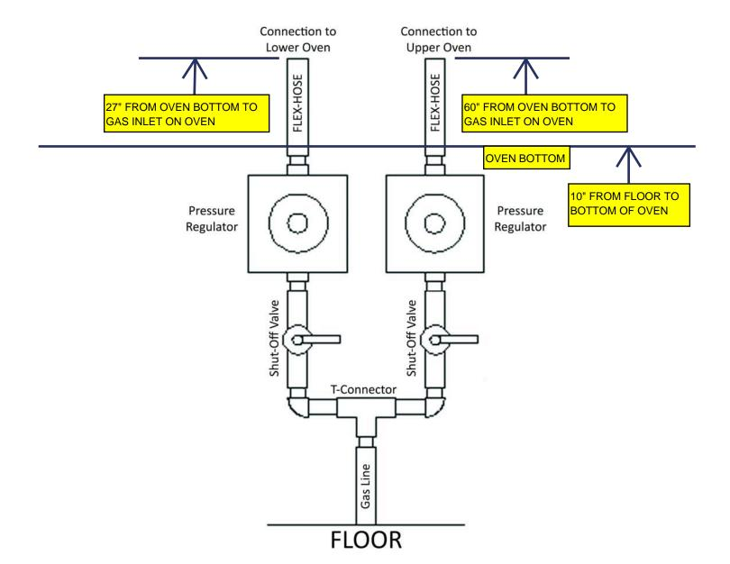
3/4" Main Gas Line should be reduced to 1/2" after the Floor. This will be connected to a 1/2" T connector using 1/2" round nipple. After the T-Connector is a 1/2" Street-L connected to Shut-Off Valve with 1/2" Round nipple, which is then connected to the pressure regulator with another 1/2" round nipple. From the top of the regulator will be another 1/2" Round nipple connecting a 1/2" (Inside Dimension) Flex hose which will run to the Oven.
