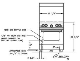
ELECTRICAL CORD LOCATED IN BACK OF UNIT LOCATION OF ELECTRICAL OUTLET MUST NOT BE HIGHER THAN 3" FROM FLOOR IF LOCATED BEHIND THE UNIT OR CAN BE LOCATED IN AN ADJOINING CABINET.
