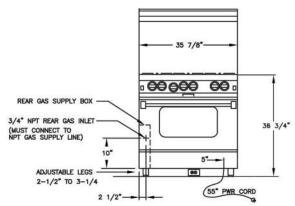
ELECTRICAL CORD LOCATED IN BACK OF UNIT LOCATION OF ELECTRICAL OUTLET MUST NOT BE HIGHER THAN 3" FROM FLOOR IF LOCATED BEHIND THE UNIT OR CAN BE LOCATED IN AN ADJOINING CABINET.
