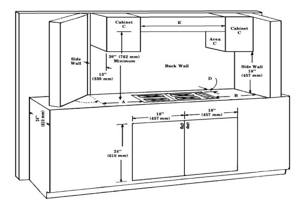
Your Drop-in Cooktop may be installed into a counter top in a row of cabinets or into an island. Refer to the illustration above for key dimensions to be followed when installing your appliance.
