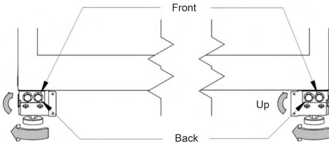
**Important:** Do not use a power drill and do not over-tighten the leveling bolts.
