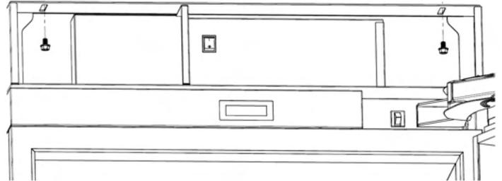
**Important:** If the mounting holes do not align with the slots in the top of the cabinet behind the top grille, it may be necessary to roll the refrigerator out of the enclosure, loosen the anchor bracket screws on the back wall, slide the bracket left or right, and retighten the screws.
