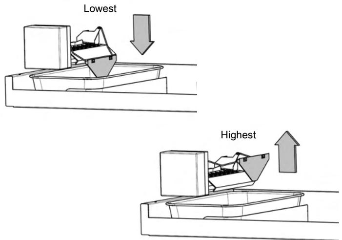
After initially connecting the household water to the water line, discard the first two full pans of ice as the ice may contain air or impurities from the water line.
