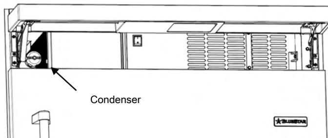
2. Use a soft bristle brush and vacuum to remove dust and lint from the condenser. Vacuum in the direction of the fins to avoid damaging the condenser.
