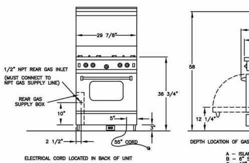
LOCATION OF ELECTRICAL OUTLET MUST NOT BE HIGHER THAN 3" FROM FLOOR IF LOCATED BEHIND THE UNIT OR CAN BE LOCATED IN AN ADJOINING CABINET.
