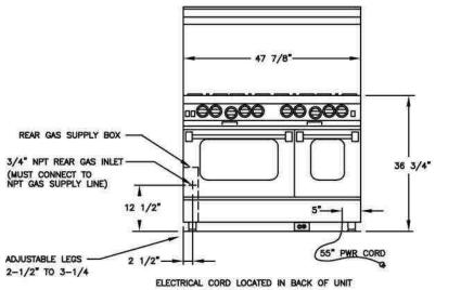
LOCATION OF ELECTRICAL OUTLET MUST NOT BE HIGHER THAN 3" FROM FLOOR IF LOCATED BEHIND THE UNIT OR CAN BE LOCATED IN AN ADJOINING CABINET.
