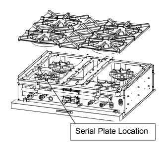
Remove the front left grate. The serial plate is on the left interior wall.
