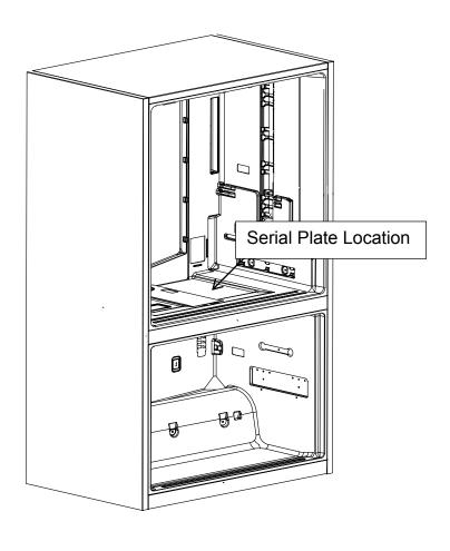
Pull out refrigerator full length deli drawer. The serial plate is located under the drawer.
