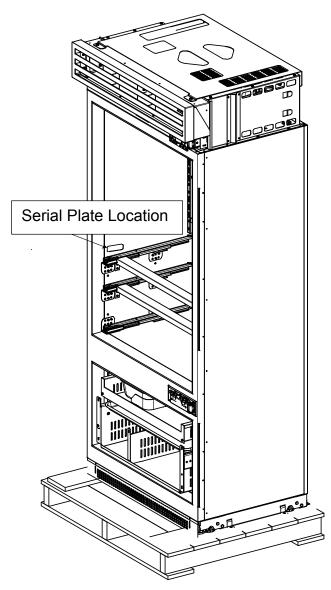
Pull out the full extension shelf. The serial plate is on the front left interior wall.
