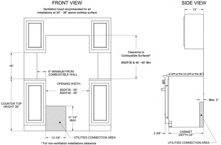
to combustible surfaces BSDF36 & 48 is 40" min
