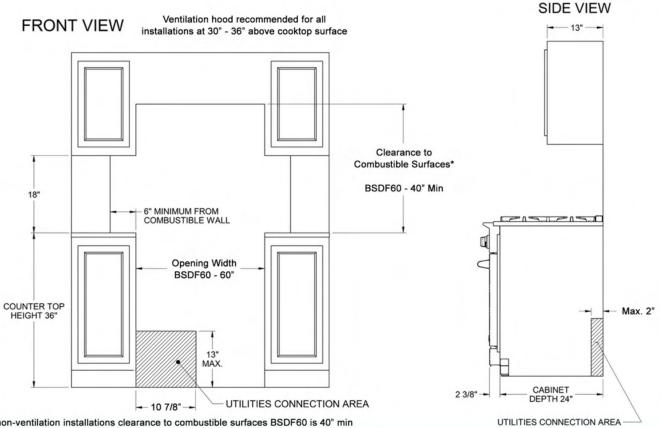
\* For non-ventilation installations clearance to combustible surfaces BSDF60 is 40" min
